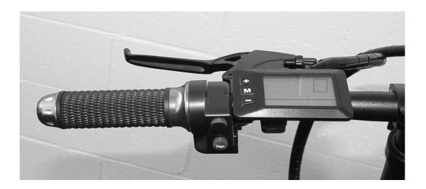
To change display settings hold the Up and Down arrows simultaneously to enter the advanced settings menu. In this menu clicking the "M" (mode) button will toggle between each Parameter setting. To adjust the value of each setting click the up and down arrows accordingly.
