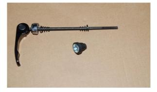
Pull out the protective cap with a little bit of force. It was there for transporting purpose.
