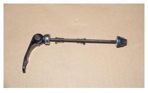
Unscrew the quick release. Notice the bigger end of spring is facing out just as pictured.
