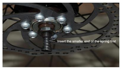
Now screw the nut to the same surface level as the end of quick release.
