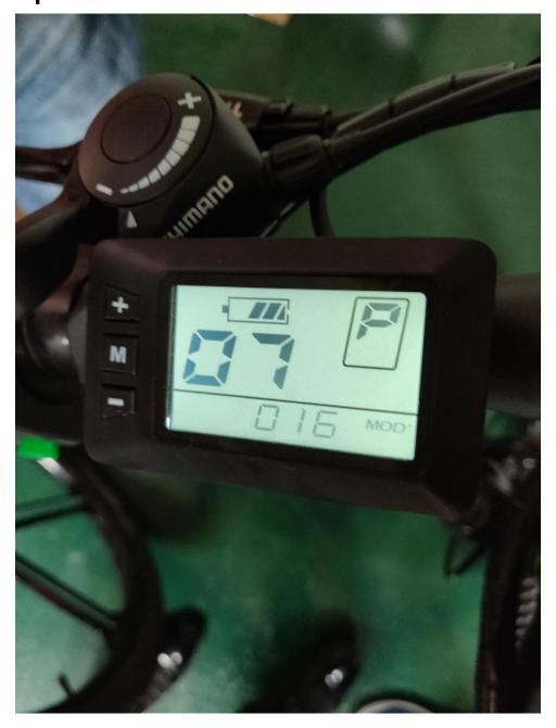
Press + or - button to change the number in the lower column of the 07 interface.
