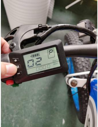
Press the + button at the 02 interface to switch between Km/h and MPH.
