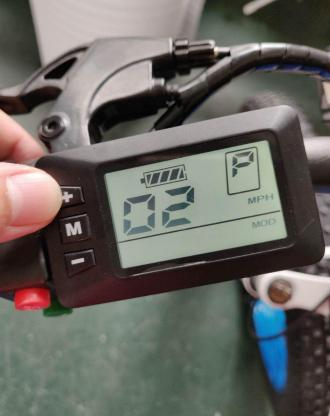
According to the above method, first press the + and - button at the same time for five seconds , and then press the M button to switch to the 07 interface.
