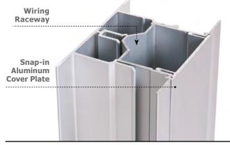
3 inch, Load-Bearing Aluminum Wiring Stud T5 temper 6063
