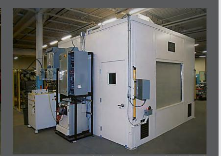
3″ 20 gauge Standard Steel System & 24 gauge Steel Faced Wall Panels
