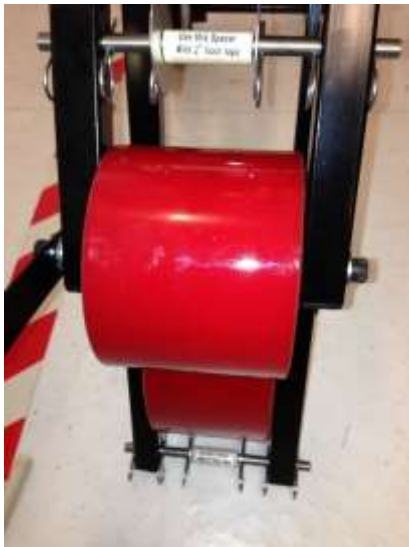
Pin and Spacer set up 2" wide tape
