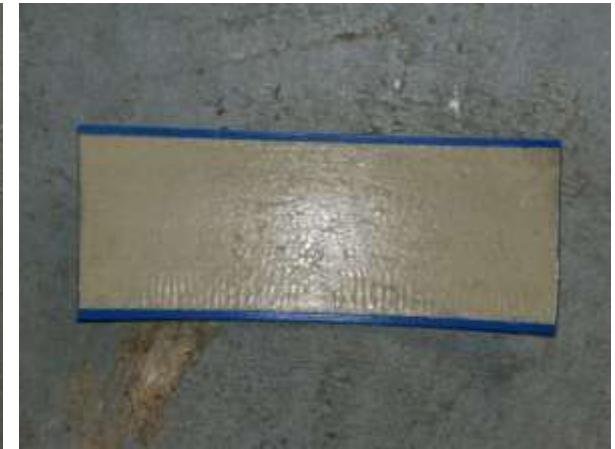
Sticky side of aisle stripe after adhering sample to the same new sealed floor. Floor was swept and scrubbed clean. Adhesion was very good. Difficulty was experience removing the sample from the floor. Note the reduction in contaminants on the adhesive.
