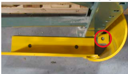
Super Duty - Three Mounting Holes See page 10
