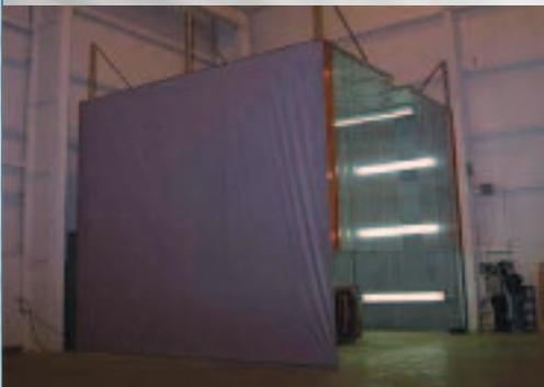
Large custom grinding booth complete with air filtration modules and overhead retractable panel to accommodate overhead crane cables and the material handling of large piece-parts.
