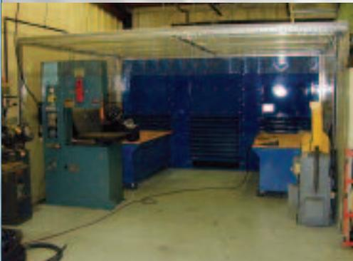
Multi-function work station: welding, grinding, touch-up spray painting, c/w cross-flow air filtration modules.
