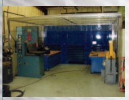
Multi-function work station: welding, grinding, touch-up spray painting, c/w cross-flow air filtration modules.
