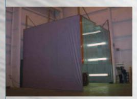
Large custom grinding booth complete with air filtration modules and overhead retractable panel to accommodate overhead crane cables and the material handling of large piece-parts.
