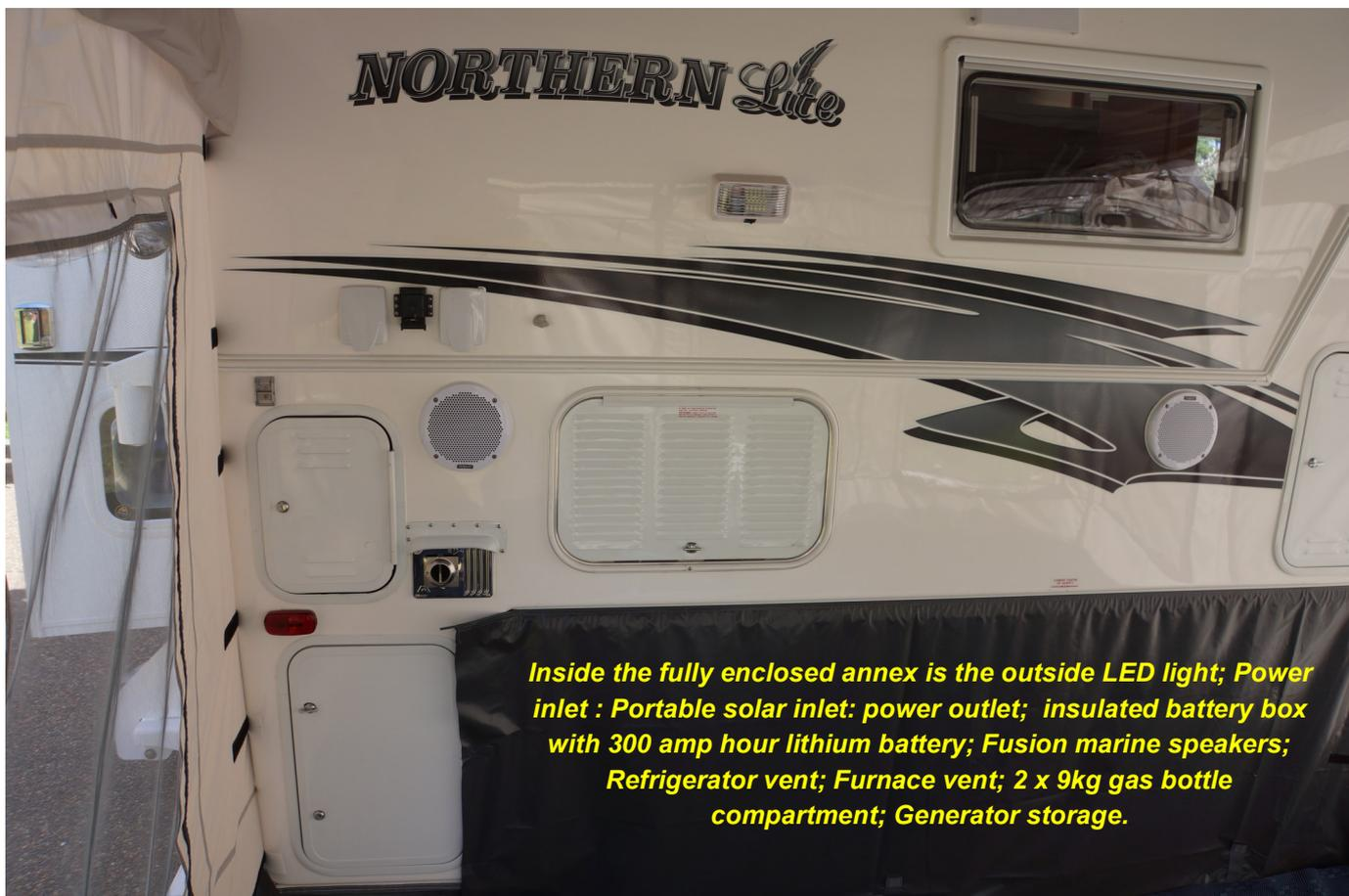
**Inside the fully enclosed annex is the outside LED light; Power inlet : Portable solar inlet: power outlet; insulated battery box with 300 amp hour lithium battery; Fusion marine speakers; Refrigerator vent; Furnace vent; 2 x 9kg gas bottle compartment; Generator storage.**
