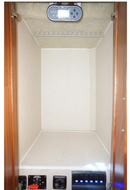
***Inside the rear robe. At the top is the Redarc BMS1230S2 remote monitor. A technically advanced system that is easy to operate. Below is the 12 volt cut off, Rear awning control and the 12 volt circuit breakers***
