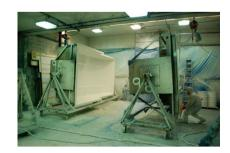
Even with the weight balanced hinges, it's a real challenge to get one of these heavy fibreglass moulds to rotate. Just to get a mould to budge, Bruce had to literally climb onto the back of a mould and use his body weight to start the mould turning. When the mould neared it's tipping point, he lowered himself down to receive the mould and put it into the proper position for gel coat or fibreglass application.
