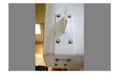
Brad also installs the jack brackets and a good number of the other external features. Here he's attaching a passenger side rear jack bracket. Note how the bracket wraps around the underside of the camper to lift the camper from the side and bottom.
