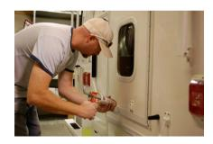
Every Northern Lite truck camper undergoes a Sealtech test before leaving the factory. During our visit, we observed Nathan install the Sealtech system, spray down the seals, and make a couple of minor seal repairs. What this means is that Northern Lite can ship these campers with full confidence that there is no break in the seals. Once the camper is in your possession, it's up to you to maintain those seals. If you do, your camper should last for many years in excellent condition.
