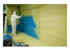
Once a set of top and bottom camper shells have been gel coated and fibreglassed, a set of insulation panels are placed and pounded into the shells. These insulation panels are built in a room next door to the fibreglass shop by Bruce Nickason. Once the panels are completed, he suits up like Bruce and Scott and sprays the panels down with adhesive. The inside of the camper shells are also sprayed with this adhesive prior to pounding in the insulation.
