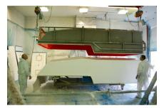
With the fibreglass shell now loose inside the mould, the team uses the hoist system to raise the mould revealing a brand new fibreglass top shell. When the team separates a fibreglass bottom shell, the technique is reversed with the top camper shell raised out of the mould. Either way, it's a spectacular show and one that's unique to fibreglass camper construction. In an instant, you can almost see half a Northern Lite camper. It may not be magic, but it's really neat to watch.
