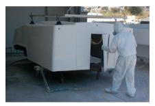
With the rough edges removed, the back door opening is cut and another hoist is attached to the top fibreglass shell with suction cups. Once the suction cups are attached, the top fibreglass shell is raised about eight feet into the air. Then the bottom fibreglass shell is wheeled under the top shell and the two shells are carefully lined up. When the shells finally see eye to eye, the top shell is lowered down onto the bottom shell.
