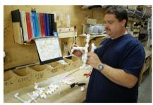
Brian Koffler is responsible for assembling the wiring harnesses and plumbing systems. Here he's holding part of a PEX plumbing assembly for a 10-2 CD Special Edition. PEX is a water supply piping system that is highly resistant to scale, chlorine, and corrosion. It's used in many brands of truck campers and is favoured for it's light weight and durability.
