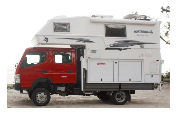
The original Aussie Base Station, was made with the Basement built on to the camper. We now build the basement onto the truck tray or even as a separate unit that can be removed from the truck if required. The drawing below gives indicates the basement as a separate unit. This configuration is lighter and allows more weight to stay on the tray when the camper is unloaded as all these trucks tend to 'ride rough' with no load. It also makes it easier to load and unload the camper.
