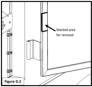
Using a Dremel or similar rotary tool, cut along the marked lines using a cutoff wheel. See figure D.3.
