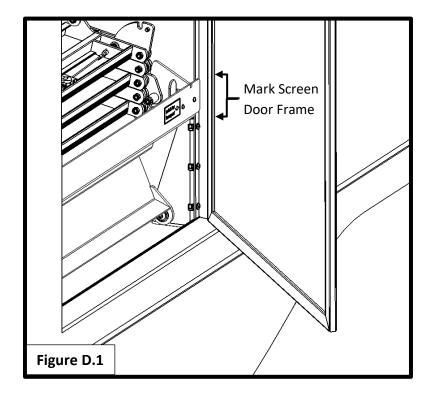
Fully open the screen door to gain better access to the marked area.  Extend the marked lines around the corners of the frame 3/16", then Connect the lines. See Figure D.2.
