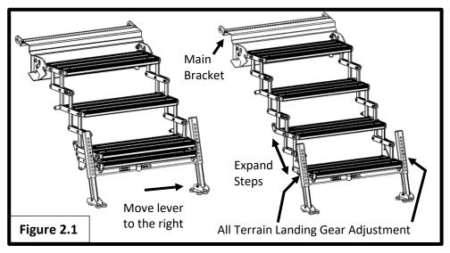
Rest the main bracket inside the door frame. If required, adjust the All-Terrain Landing Gear to allow the main bracket to sit against the floor inside of the threshold molding.
