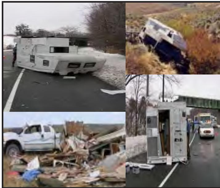
The design of the slide-in is extremely important. The center of gravity and the location of storage compartments are critical. When turning a ‘normal’ corner and the unit ‘heels’ more than 5 degrees—which isn’t much—you should be asking yourself, “What can I do to correct it?” If passing trucks or sidewinds cause an uncomfortable ‘sway,’ you should be asking yourself, “What can I do to correct it?” Then, if it can’t be corrected, you should be considering the risk of continued use.
