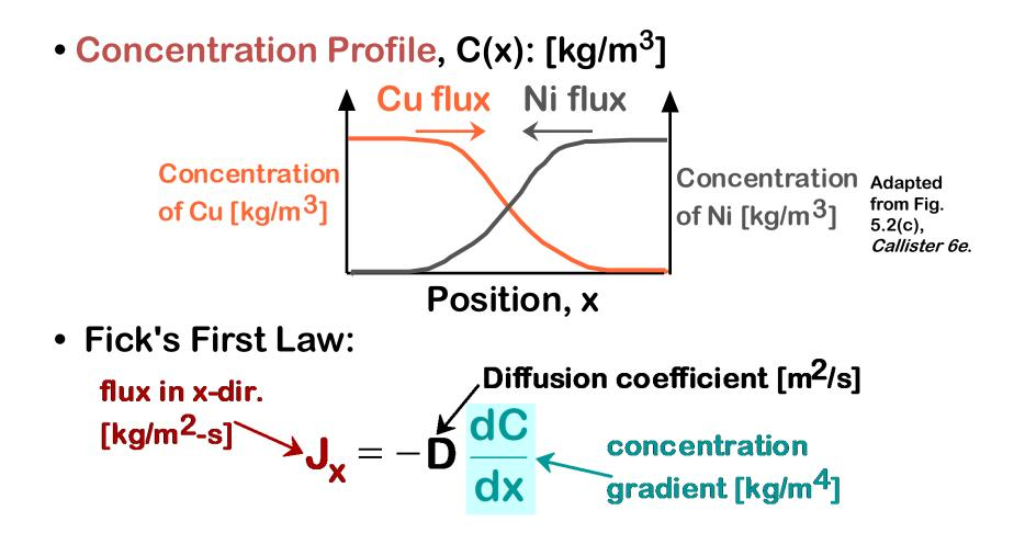
The steeper the concentration profile, the greater the flux!
