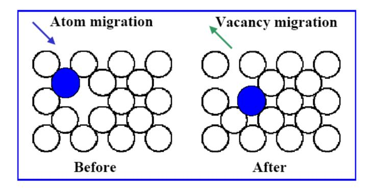
Energy is needed to generate a vacancy, break bonds, cause distortions. Provided by HEAT, kT ! Atom moves in the opposite direction of the vacancy !
