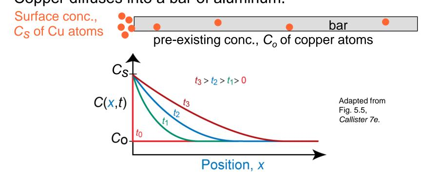
B.C. at t = 0,  $C = C_o$  for  $0 \le x \le \infty$ at t > 0,  $C = C_S$  for x = 0 (const. surf. conc.)  $C = C_o$  for  $x = \infty$
