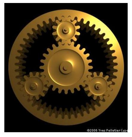
It is the system of epicyclic gears in which at least one wheel axis itself revolves around another fixed axis.
