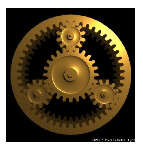
Planetary gear trains have several advantages. They have higher gear ratios. They are popular for automatic transmissions in automobiles. They are also used in bicycles for controlling power pedaling automatically manually. They are also used for power train between internal combustion engine and an electric motor.
