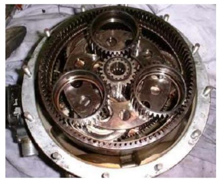
This design can produce large gear ratios in a small space and are used on a wide range of applications from marine gearboxes to electric screw drivers.
