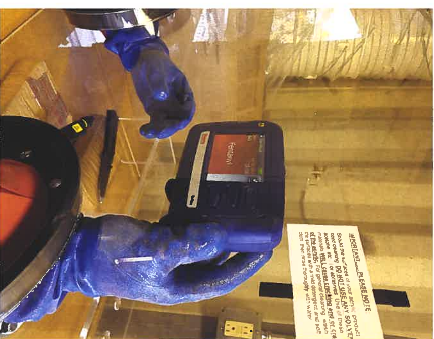
One of many devices used in the field to detect contraband, this TruNarc substance analyzer identifies multiple types of narcotics. The gloved manipulators protect officers while testing for drugs. Photo courtesy of CBP NTC
