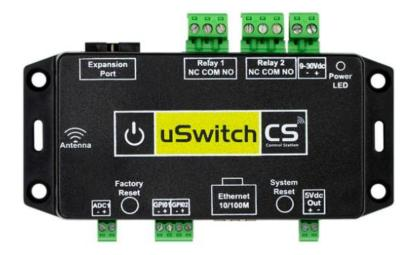
**What it is:** Expandable 2 Channel WiFi IP Relay and I/O controller to manage, sense, automatically reboot, and control any device, anywhere, anytime over LAN/WAN from any iPhone, Android, PC, or MAC.
