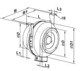
Typical Fan for 400i is a pre-wired 3 prong plug VKM 250 fan, 2 Fans needed.
