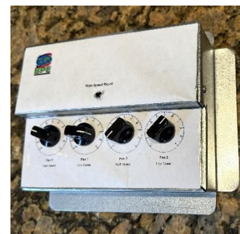
BPE Forex Controller—front panel with four speed dials and High-Speed Reset button.
