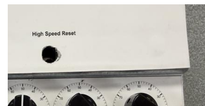
High-Speed Reset button starts the 20-minute boost.
