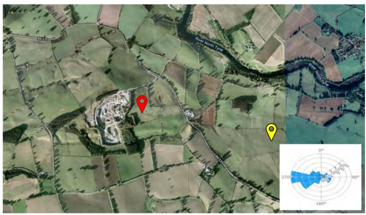
Site Plan with suggested turbine location (red pin & yellow pin)
