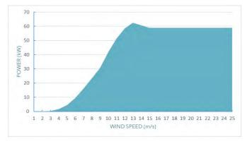
\* Indicative power curve and estimated energy output. Based on ongoing testing.
