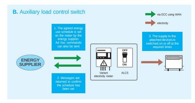
HCALCS – HAN connected ALCS - operate in a similar way to a regular ALCS, this allows switching of a remote load via the HAN network. For example, this functionality could be implemented in an electric vehicle charger.
