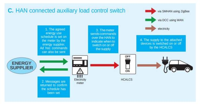
• ALCS switching is currently a binary on or off output, however current draft SMETS specification also detail a proportional control mode – where a load can be modulated between 0 and 100% via a control signal.
