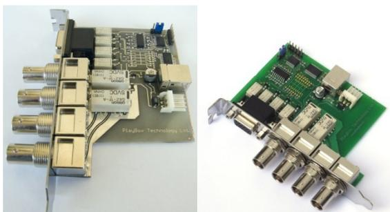
The PlayBox GPI Relay board has **4 GPI Inputs, 4 GPI Outputs with Relays, 1 Bypass relay (up to 2.6GHz)**
