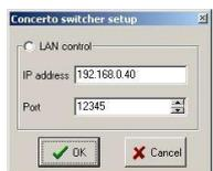
The configuration dialog represents the *LAN* setup for controlling Concerto switchers. Fill in the *IP address* and *Port number* of the switcher and click **OK**.
