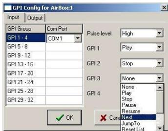
The column to the left contains a list of **GPI Groups** (four different GPI pulses per COM port). The *GPI 1* stands for the CST pulse (input on pins 8 and 5), the *GPI 2* is DSR (pin 6 and 5), the *GPI 3* is RI (pin 9 and 5), and the *GPI 4* is CD (pin 1 and 5).
