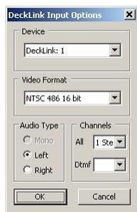
This plug-in allows for reading DTMF tones, embedded in an SDI video signal, or coming through the analog audio inputs of a *Blackmagic DeckLink board*. Select it in the plug-ins list and click **Assign**.
