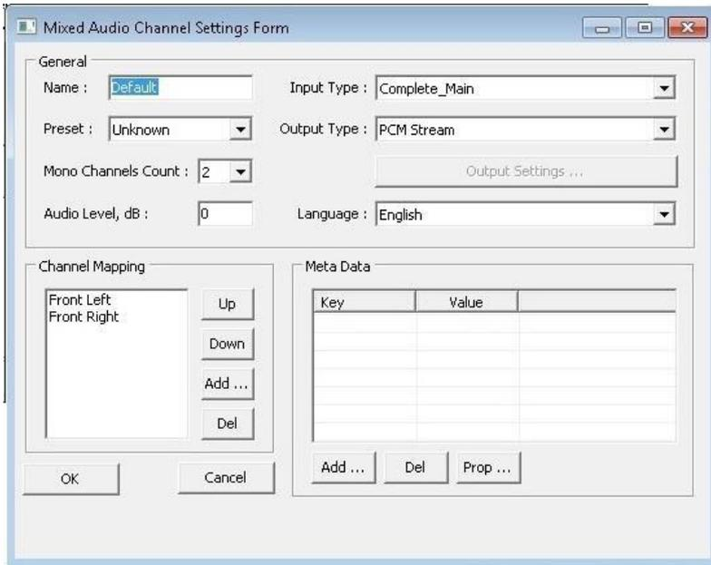
EXAMPLE: If you select **Stereo**, the channel mapping will contain a [Front Left] and a [Front Right] channel. If you select **3 front LFE**, there will be: [Front Left], [Front Right], [Front Center], and [LFE Subwoofer].
