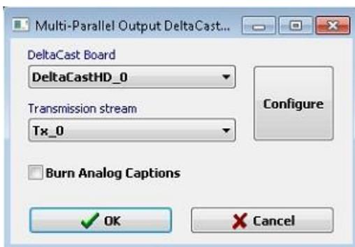
Select the Deltacast board and Transmission stream in the Setup dialog. Check Burn analog captions to enable this option.
