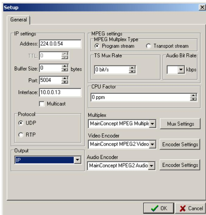
will have to enter a special multicast address in the **Address** field (the multicast addresses are in the range between 224.0.0.0 and 239.0.0.0).
