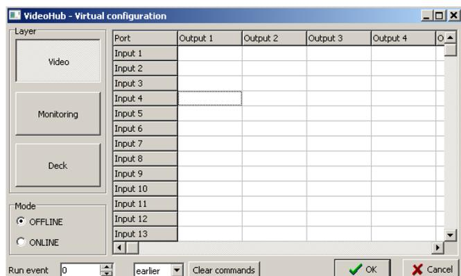
This event activates the **VideoHub Switcher**. Before adding/inserting such an event, you need to configure its settings from [Settings > Modules > Remote control > VideoHub Switcher Output](#).
