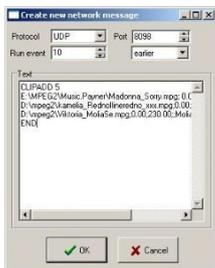
The Net Sender Output event will send any text message via UDP. Thus, you could control IP-enabled third-party devices. All you have to do is specify the port, to which the message will be broadcast and type in the text. **AirBox** will send the message on the specified port when it reaches the event line in the playlist, observing the offset (if any).
