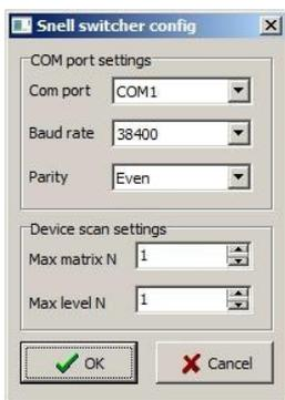
This is an external plug-in used to control Snell devices that comply with the *SW-P-08* protocol. It uses *RS-485* cables. The COM port settings may vary for different devices.
