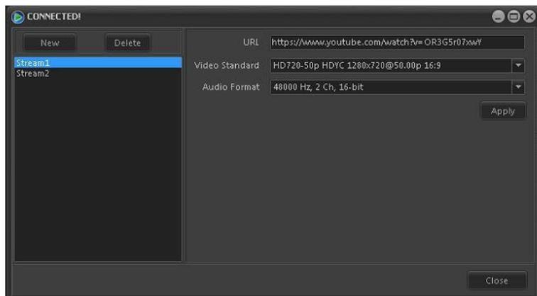
All existing input stream presets are shown in the pane on the left. The right pane contains the stream configuration options for the selected preset.
