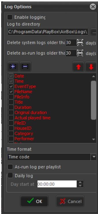
**AirBox** generates two types of log files: System logs and an As-Run log. A *Logs* directory is created upon **AirBox** installation. It contains a *System* subfolder by default. *Errors*, *System events*, *Events*, and *Event type* are logged in the *System log*, regardless of your preferences.
