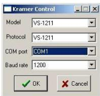
The **Kramer Switch** module allows you to control all x01 and x11 Kramer Switchers. **AirBox** controls them via the old protocol only. Protocol 2000 is NOT supported in this plug-in! The switchers may be controlled via *RS-232* and/or *RS485/422* communication ports.
