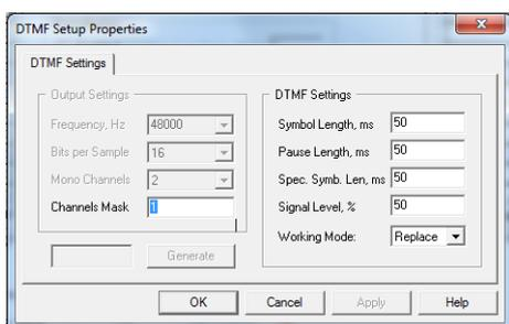
Under *Output settings*, define the parameters of the DTMF tone – *Frequency*, *Bits per sample*, number of *Mono Channels*, and *Channels Mask*.
