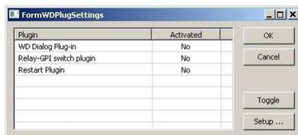
The **WatchDog** Plug-in detects if some malfunction of the application occurs. When a malfunction takes place, **WatchDog** runs “activated” Sub-Plug-ins from its sub-Plugin list
