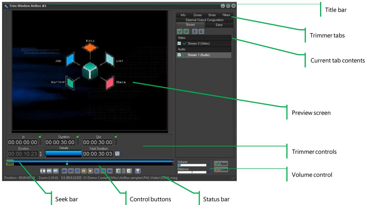
The **Clip Trimmer** combines a VGA preview screen and tools for editing the *In* and *Out* points of *MPEG* clips.
