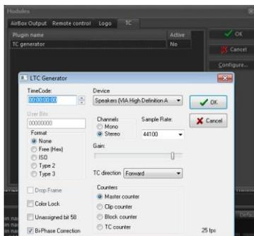
Above you can select the output *Device* and set the output channel type and sampling rate.
