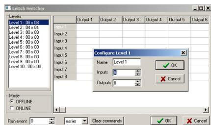
This is another optional plug-in for **AirBox**. When you choose to insert a *Leitch Matrix event*, the dialog to the right is displayed. Double-click on the relevant level to configure it (i.e. to specify the number of inputs and outputs in it) and click *OK*.
