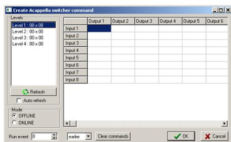
This is an event for controlling an external video/audio router. Depending on the switcher model, the currently available inputs/outputs will be displayed in a matrix grid, in which you can configure the command you need. Click **OK** when ready. You can also set an event offset via the *Run event* field, if necessary. The number you enter in the field is in milliseconds.
