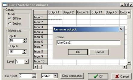
As in all other switcher events' properties, you can rename the Inputs and Outputs in the interface for easier navigation. For renaming, just double-click on the Input/Output and type the new name.
