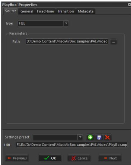
The **Source** tab contains a basic clip description. Select the type of *Type* fields shows whether the input is from a **File**, a **Live**, or a **UDP** source.
