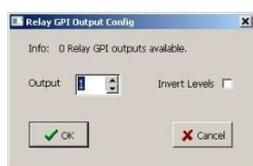
The **Relay GPI Output** is performed via dedicated [output events](#) in the playlist. When the playback reaches the event, the Relay GPI trigger is activated.
