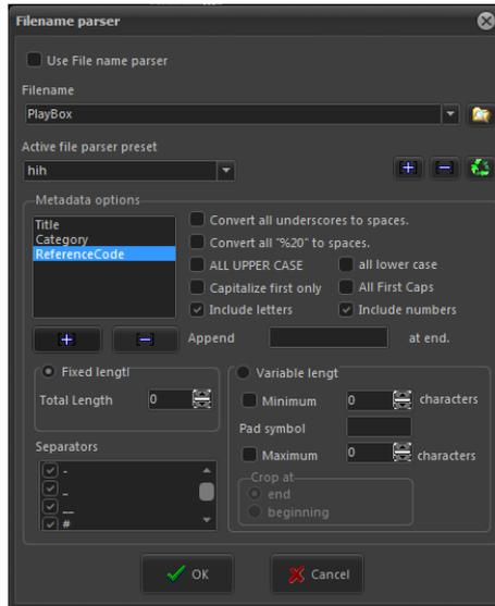
This module will allow **AirBox** to Parse names of files and get information from them. It provides an easy way to use information, included in the file name, without using a database. You can make the most of this feature if you have a standard naming structure for your clips.
