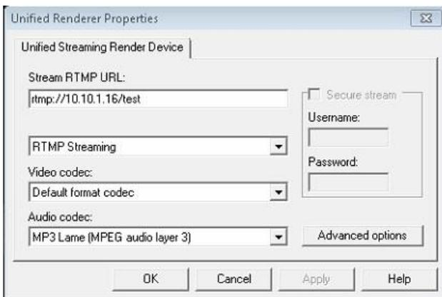
In the *Stream RTMP URL* field, enter the address to which you want to stream. The URL must be entered in the following format: **rtmp://address/location**.
