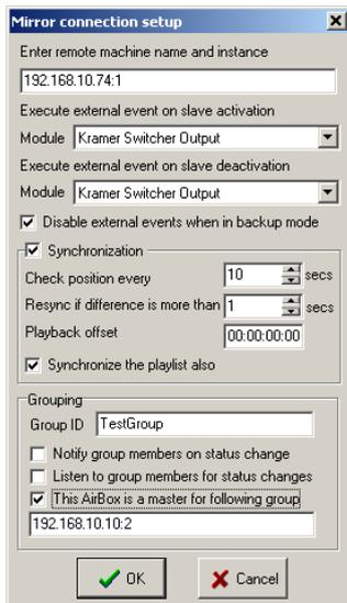
The **Mirror mode** is another optional plug-in, available for **AirBox**. The Mirror mode provides options for full redundancy of your main playout unit against system failures, such as power loss, broken motherboard or RAM, etc. In order to use this option, you must have two licenses for **AirBox**, running on two different workstations with a network connection between them. For the sake of convenience, these are called *Master* and *Slave* hereafter. They communicate via TCP/IP protocol.
