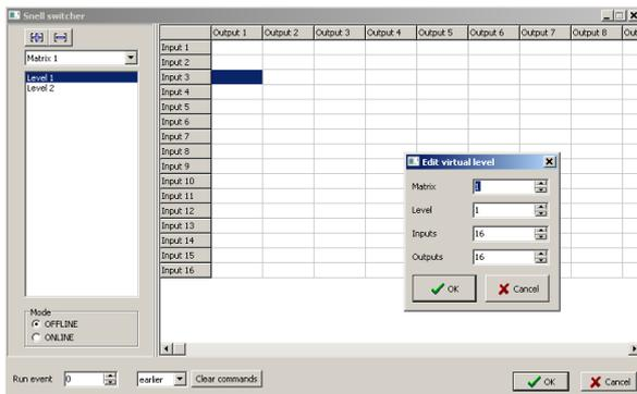
This optional plugin is used to control Snell devices that comply with the SW-P-08 protocol. It uses RS-485 cables. COM port settings may vary for different devices. The matrix is configured in the same way as the Sierra Video Switcher event's one above. The only difference is that here you can set more than one matrix, in case you have more than one device.
