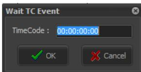
Automatically stops the playback and resumes it upon reaching the specified time code (e.g. coming from an external timecode generator). The message to the right will be displayed on the **AirBox** window and the Master counter will continue running. See the [LTC reader description](#) in the **Settings** menu > **Timecode** section further in this chapter.
