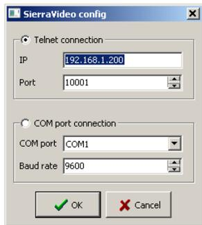
Clicking the **Configure** button while the **SierraVideo Switcher Output** row is selected will evoke a setup dialog, where you can setup the connection to this switcher. You can select from two types of connections:
