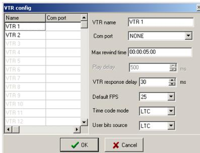
You can use it to control up to two VTRs for combined file-based/tape-based playout. Enable it and click **Configure**. A dialog will open for you to make the necessary setting. First, enter the **VTR Name** and the **COM port**, to which it is connected. Then, specify the maximum rewind time. Please, note that in the playlist you do not have to insert VTR events that are overlapping in relation to the maximum rewind time!
