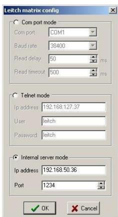
**AirBox** can control Leitch Matrix Switchers either through the computer COM port or using the IP address of the matrix (via TCP/IP protocol). The configuration window is divided into three areas – one per each mode.
