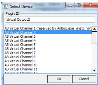
**Virtual Outputs** can be used for streaming. Virtual outputs, defined from this dialog box will be displayed as **MPO Video Capture source** in most video players that support such functionalities and can be previewed locally.
