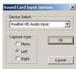
This plug-in is to be used for analog audio tones, received on your PC sound card (coming from an IRD, for example). Select this line and click **Assign** to load it. Then, click **Configure** to select the sound input device and configure it:
