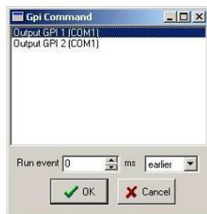
Inserts a line in the playlist, which activates the **GPI Output**. A dialog box appears to define the output **GPI** commands. You can have up to two commands on each COM port: GPI 1 means DTR tone (pulse on pin 4 and 5), and GPI 2 means RTS tone (pulse on pin 7 and 5).
