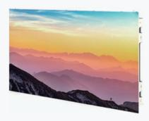
The box structure adopts high strength sheet metal sandblasted iron box with unique segmented splicing technology. Effectively reduce the splicing gap of the screen body
