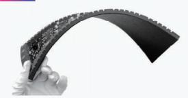
PCB board adopts flexible soft board, bottom shell adopts silica gel material, which has good flexibility and eliminates static electricity
