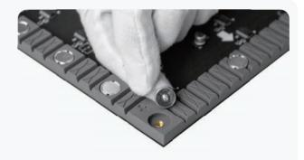
The PCB board uses copper column welding and back glue to form a lockable iron base with the bottom shell, which makes the module more solid and reliable
