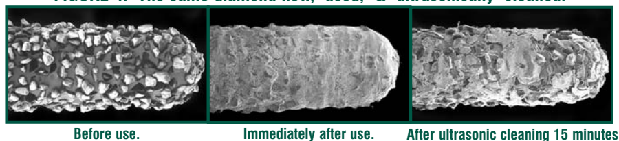
FIGURE 4. The same diamond new, used, & ultrasonically cleaned.
