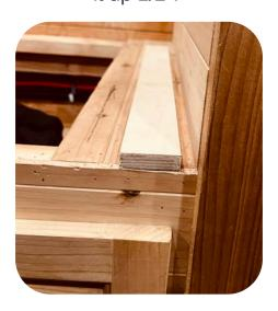
**Step 12.** Place your provided 1/2" shims in the location that you marked in the second step. Now place your sofa on top of the 1/2" shims and screw it back down where it was originally located.
