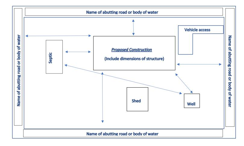
The arrows in this example show the distance measurements you must include on your site plan and footprint drawing that you are required to create on page 4.
