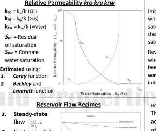
Unsteady-state 2. (Transient) flow  $\left(\frac{\partial \mathbf{p}}{\partial t}\right) = \mathbf{f}(\mathbf{i}, \mathbf{t})$ Pseudosteady-3. state flow  $\left(\frac{\partial p}{\partial t}\right) = constar$
