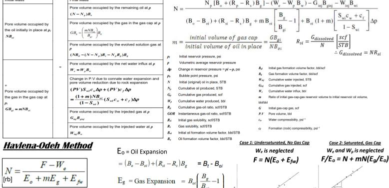
$E_{\text{fw}} = (1+m)B_{oi} \left[ \frac{c_w S_{wi} + c_f}{1-S} \right] \Delta p$ where  $\Delta p = p_r - p_r$
