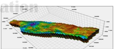
The reservoir formation 3D grid was divided at an optimum of 100m2 blocks. This qualifies the grid as Coarse Grid, thus enabling a fast and efficient simulation run as a result of the reduced volume in calculations required to complete the simulation. The target reservoir formation was evaluated from depth 4000m to 5200m.
