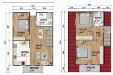
Ground floor plan 74m 2 +5m 2 Veranda=79m 2 1st floor plan 50m 2 +5m 2 balcony=55m 2
