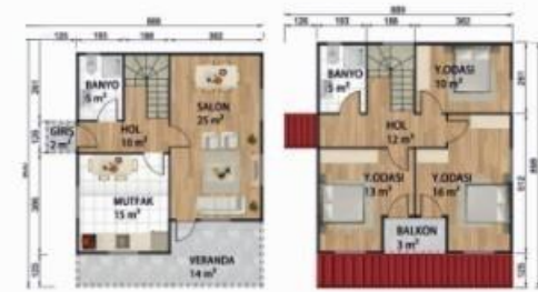
Ground floor plan 57m 2 +14m 2 Veranda=71m 2 1st floor plan 56m 2 +3m 2 balcony=59m 2
