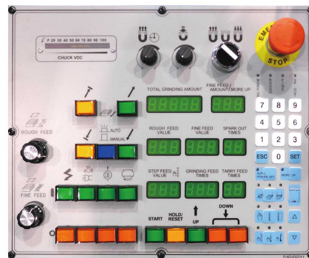
AUTOMATIC DOWNFEED AD5 (NC) CONTROL PANEL (optional)
