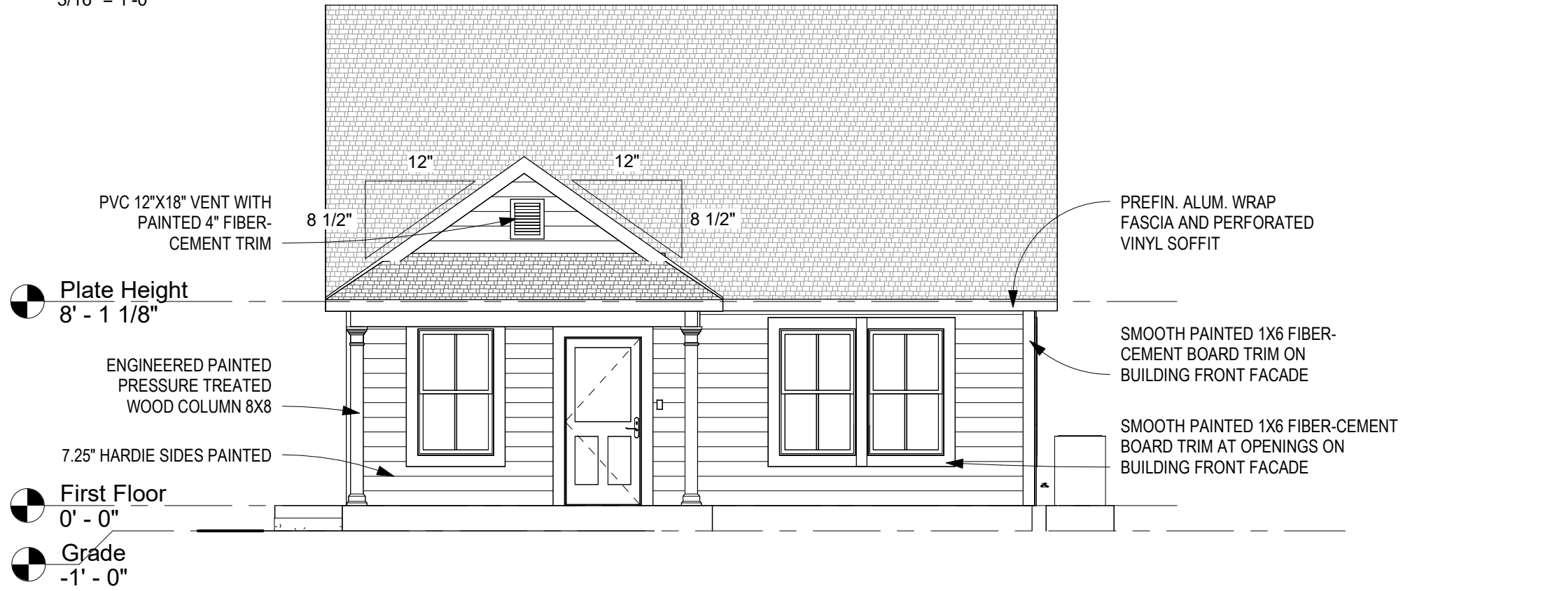
1 Front Elevation Verion 3 A200 3/16" = 1'-0"
