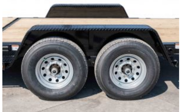
8 Lug 7K Axles – 235/80 R16 Premium West Lake LRE Tires – Slipper Spring Suspension
