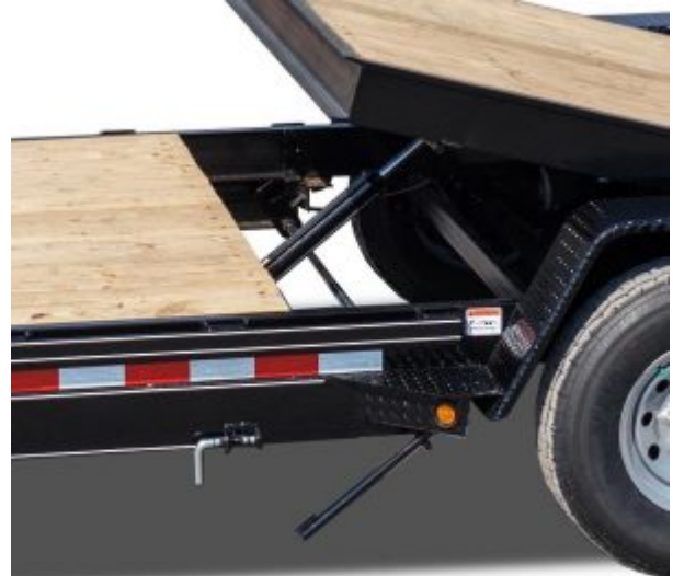
Damper Cushion Cylinder For Controlled Lowering of Tilt Bed
