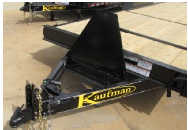
Tool Box With Lockable Lid – Heavy Duty Cast Iron Adjustable Coupler.
