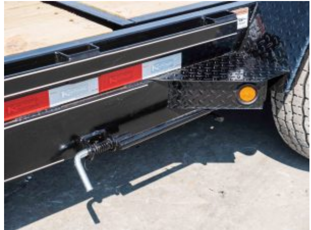
One Handle Latch To Lock Down Or Release Tilt Bed With Spring Loaded Lock
