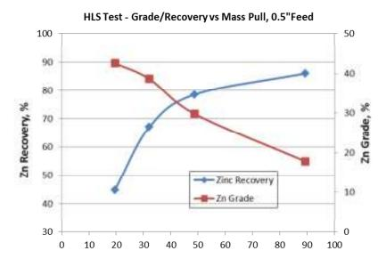
FIGURE 13-6 Zn RECOVERY & Zn GRADE vs. MASS RECOVERY, ½ INCH FEED
