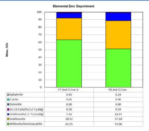
FIGURE 13-10 ELEMENTAL ZINC DEPORTMENT OF CONCENTRATE FROM TEST F7 AND F8
