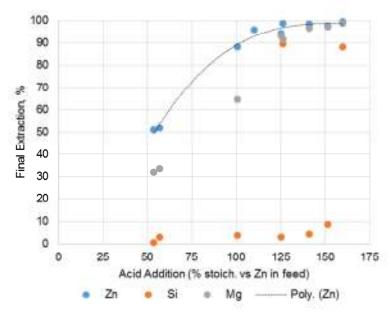
FIGURE 13-12 KEY METAL EXTRACTIONS vs. ACID ADDITION
