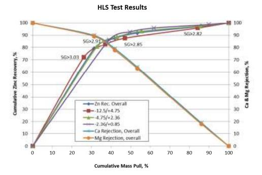
FIGURE 13-4 MASS YIELD -Zn RECOVERY & Ca, Mg REJECTION
