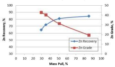
HLS Test - Grade/Recovery vs Mass Pull, -14 M Feed
