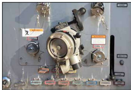
Figure 9.28 An intake pressure relief valve.
