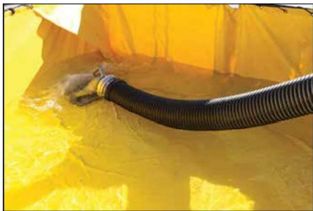
Figure 10.20 Use a low-level strainer when drafting from a portable tank or swimming pool.
