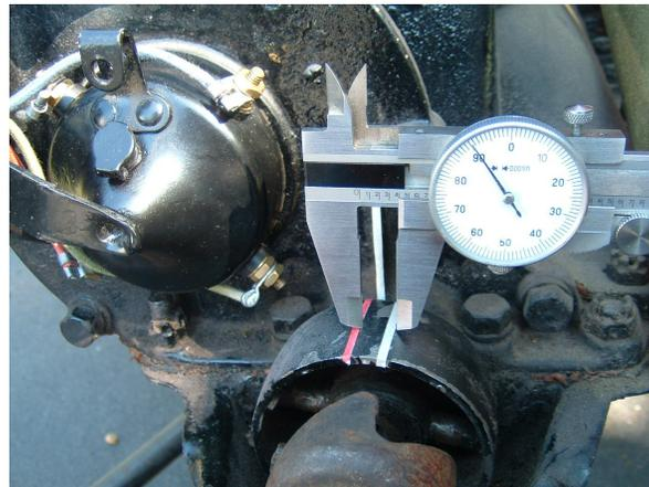
**Figure 7.** Measuring the crank travel between cylinder 1 TDC and cylinder 1 firing position.
