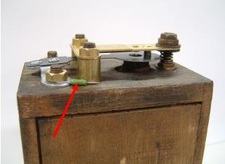
Figure 4A – Adjacent under point terminals Loosen nuts and slip fuse jumper wires Under point mounting posts.
