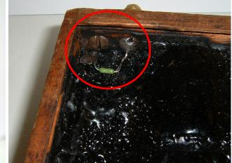
**Figure 4C** – Internal, clear tar and solder Across point post terminals. Completely Hidden from view for undetectable install.
