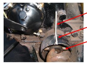
Use masking tape to mark reference line on timing cover
