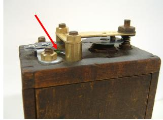
**Figure 4B** – Hidden under vibrator spring Under silver and brass point terminal posts.
