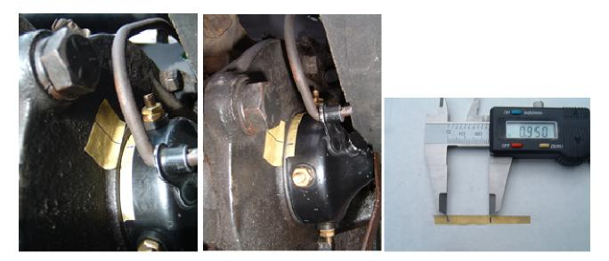
A. Spark Lever Fully Retarded B. Spark Lever Fully Advanced C. Measure Rotational Travel
