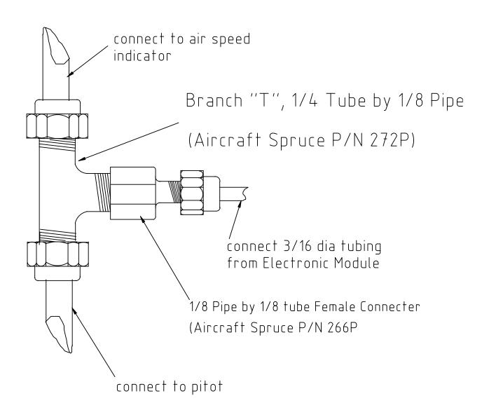
Cut existing pitot tube, and install fitting as shown. Side connection should contain a restrictor to prevent airspeed loss in the event of air leak.
