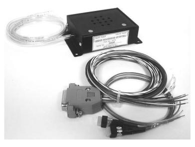
that mount on the instrument panel. One switch-light is labeled for water landings and the other switch-light for runway landings. The unit is interconnected to existing or user-provided landing gear position indicating lights, a user-provided landing flap position switch, the pitot system and the aircraft audio panel, VHF transceiver or pilot headset jack. Audible voice warnings are heard in the pilot headset and through the small internal Gear Alert speaker.
