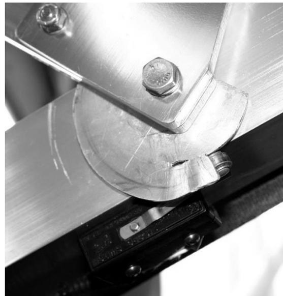
The ACI “e-Flaps” Flap Controller also provides a constant ground for the 2080 Gear Alert when flaps are in the landing position.
