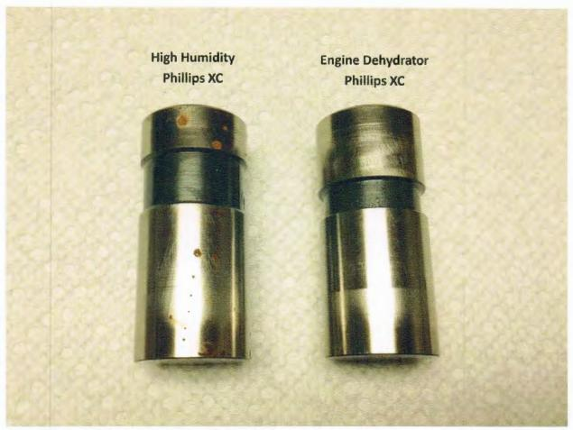
After 24-days, the lifter cooked in Phillips XC engine oil had significant rust and pitting on most of its surfaces. The top quarter of the lifter was much worse than the bottom as clearly, the oil drains off the lifter from top to bottom over time. The other lifter cooked in Phillips XC, but alternatively placed in the low humidity chamber had no sign of rust.
