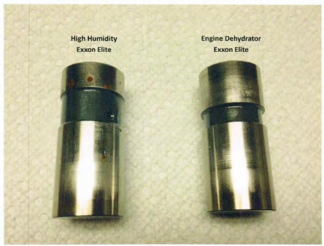
After 24-days, the lifter cooked in Exxon Elite engine oil had small patches of rust to the top third of the lifter body, only. The other lifter cooked in Exxon Elite, but alternatively placed in the low humidity chamber shows no sign of rust.
