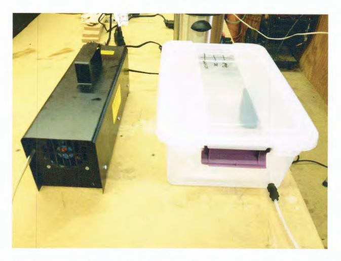
The second humidity chamber used a high-flow humidifier that produced a measured range of relative humidity from 85-93 percent.
