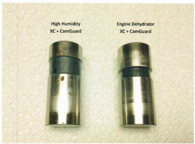
After 24-days, the lifter cooked in Phillips XC engine oil plus CamGuard anti-corrosion additive had rust on the top third of the surface, and some minor signs of rust on the lower body. The other lifter cooked in Phillips XC + CamGuard, but alternatively placed in the low humidity chamber had no sign of rust.
