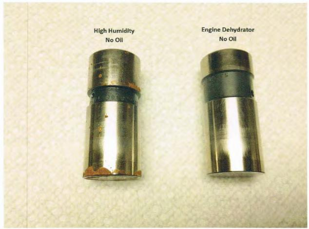
After 24-days, the lifter baked in the oven with no oil coating had heavy rust and pitting on all surfaces. The other lifter baked with no oil but alternatively placed in the low humidity chamber had no sign of rust.
