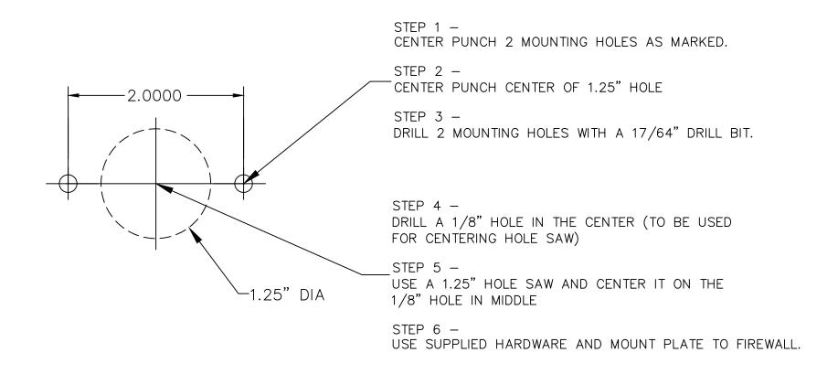
6AN / 8AN FIREWALL NITROUS BULKHEAD
