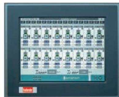
Touch screen operator interface for up to 16 gravimetric feeders
