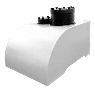
CarboPack BT is an instrument that performs measurements of carbon dioxide permeability for accurate shelf life forecast useful in the beverage and general packaging (bread, cheese, coffee, etc) applications.
