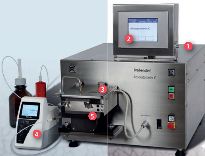
Absorptometer "C" with mixer for testing carbon black
