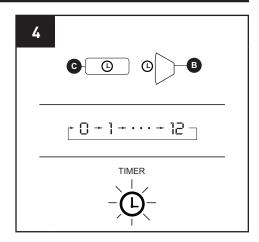
To set the timer power on, while powering off the unit press the Timer button on the control panel (C).
