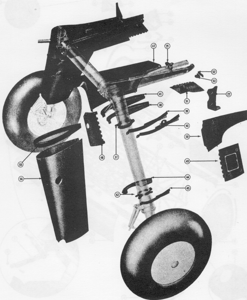
Figure 18—Fuselage Cowl Installation (Sheet 2 of 2 sheets)
