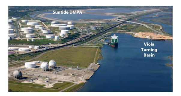
On the Inner Harbor almost all of the land on the north side of the channel was created through the beneficial use of dredge material from the original channel construction, channel deepening, subsequent levee construction and maintenance dredging.
