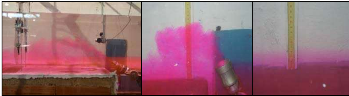
Fig. 4. Physical model test of a brine single jet discharge. Figure 4A shows the jet flow path in the near field region. Figure 4B) shows a detail of the jet orifice and flux exit. Figure 4.C) shows the brine hypersaline plume which is typical of the far field region.
