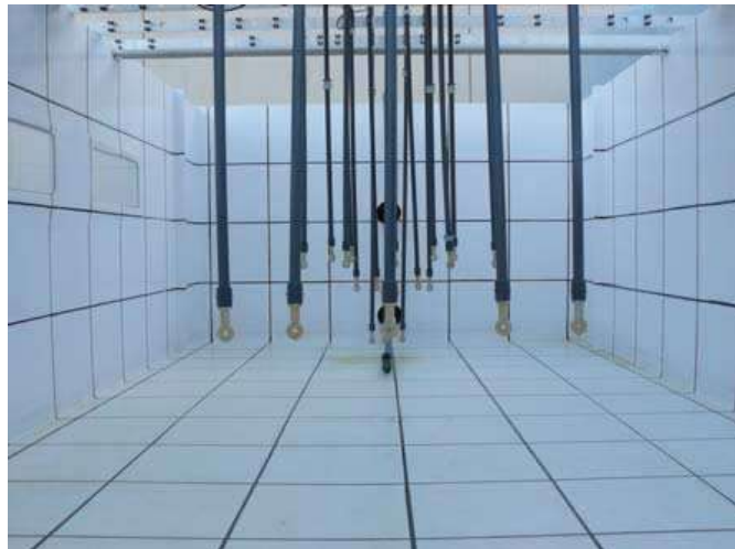
Fig. 5. Tank and gauges for brine discharge physical experiments.
