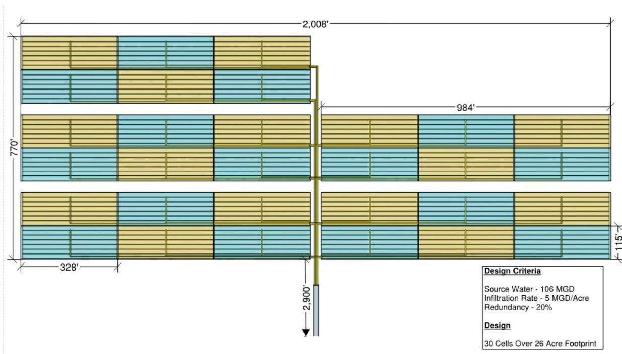
**Figure 4. Schematic of proposed SIG design at Huntington Beach.**
