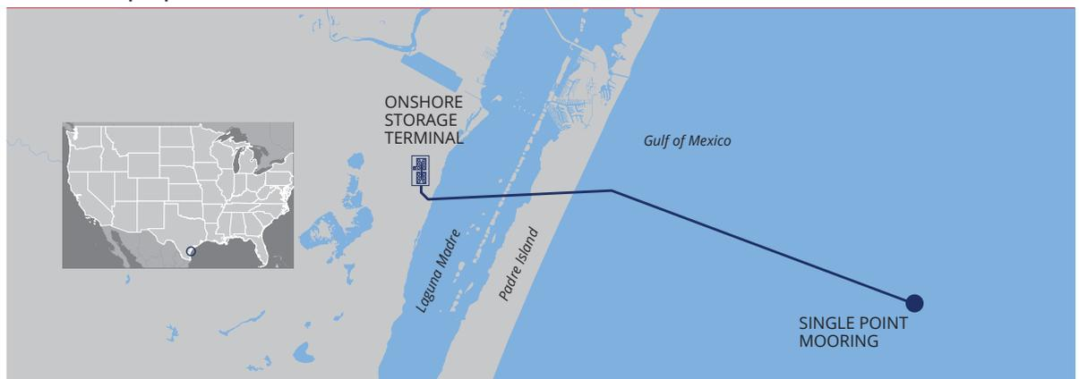
As described above, the SPM will be located approximately 14.7 miles off the coast of North Padre Island and anchored to the seabed using a symmetrically arranged six-leg anchor chain system that extends to anchor piles on the seafloor. The SPM will have a rotating table that allows the vessel to safely float around the buoy during loading operations and utilizes a PLEM system to connect the subsea pipelines to the SPM.
